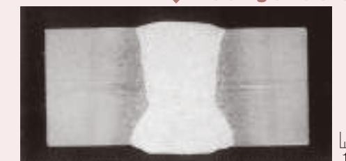
Example of large heat-input welding joint (1 pass, heat input 150 kJ/cm)
