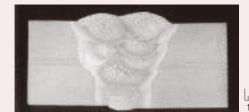
CO 2 shielded gas welding method (7 passes, heat input 30 kJ/cm)
