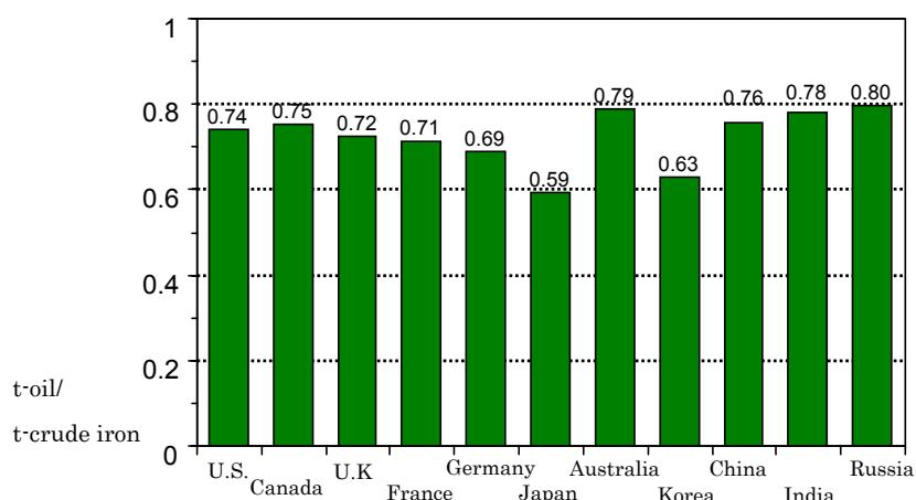
Japan ranks higher than the U.K., Germany, France and all other countries in terms of energy efficiency at integrated steel mills. Japan's leadership is due in large part to the extensive use of exhaust heat recovery equipment and the high utilization rate of byproduct gases.
