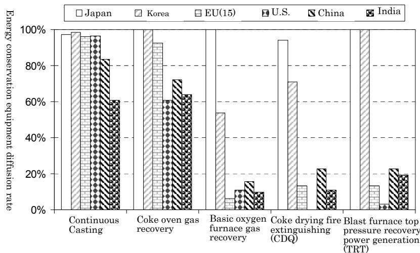
The diffusion rate of exhaust heat recovery equipment (CDQ, TRT) is much higher in Japan than in Europe and the U.S. Furthermore, Japan is clearly ahead of other countries in the recovery of byproduct gases (coke oven gases and basic oxygen furnace gases).
