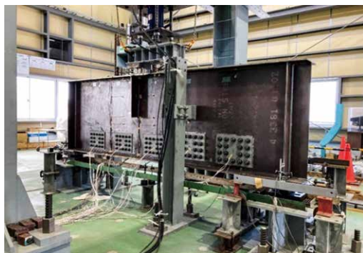
Photo 1 Four-point bending test specimen
