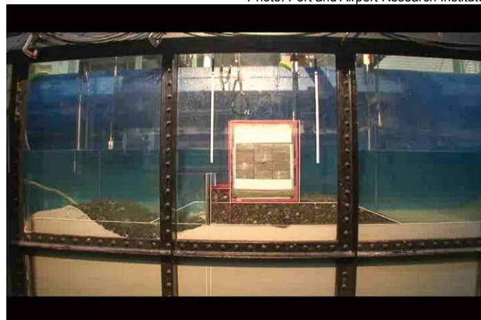
Photo1 Scouring of the ground behind the breakwater reinforced by the use of steel pile
