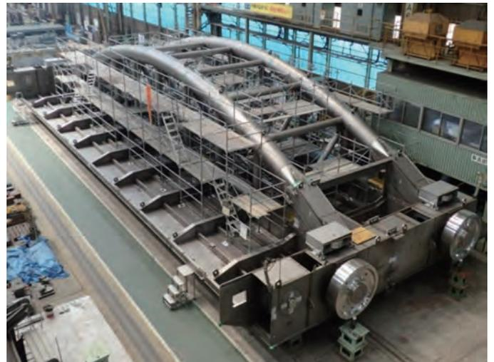
Photo 2 Temporary assembly at fabrication plant
