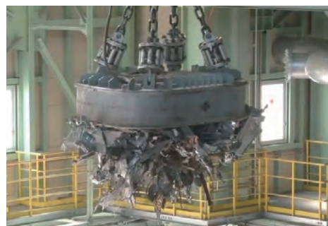
Photo 1 Magnetic separation of used steel products from waste materials Photo: The Japan Iron and Steel Federation
