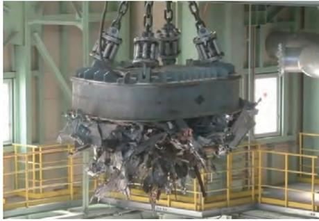
Photo 1 Magnetic separation of used steel products from waste materials
