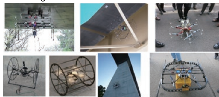
Fig. 3 Drones Being Developed in SIP for Inspection of Bridge Girders and Piers
