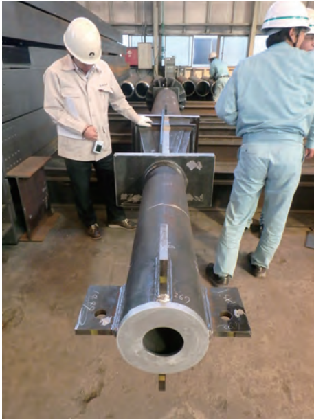
Photo 5 Heavy-wall seamless steel tube used as column
