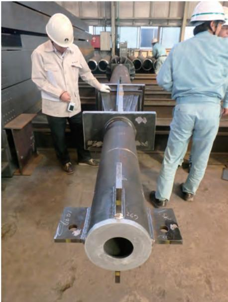
Photo 5 Heavy-wall seamless steel tube used as column
