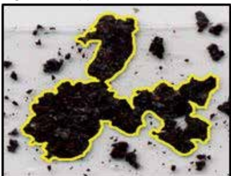
Fig. 3 Overlapped Rust Particles
