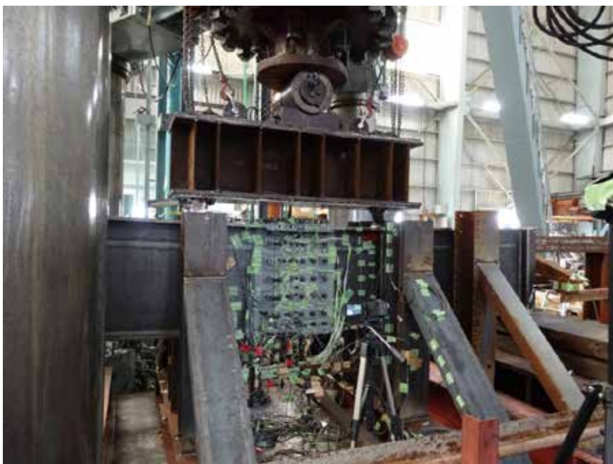
Photo 2 Flexural bending test for I-girder bolt joint
