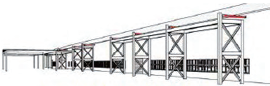
Fig. 6 Response-control Buttress Framing Installed Outside of Plant
