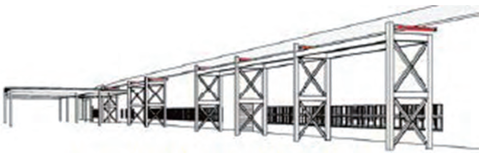
Fig. 6 Response-control Buttrass Framing Installed Outside of Plant
