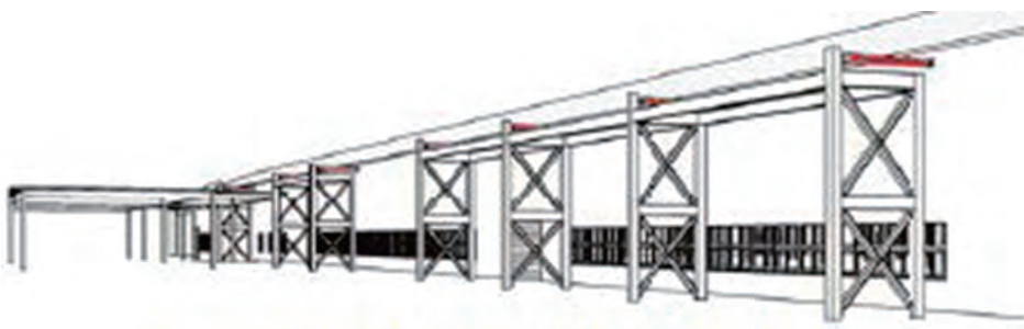
Fig. 6 Response-control Buttrass Framing Installed Outside of Plant
