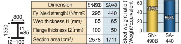
**Table 3 Features of TMCP Steel in Mechanical Properties**
