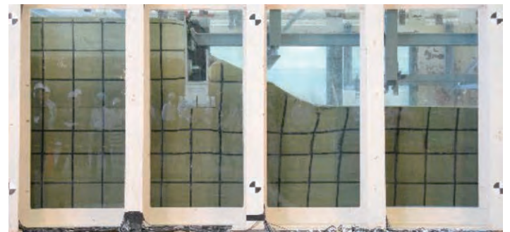
Photo 3 Ground deformation after excitation (Case 1)
