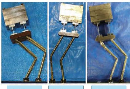
Photo 2 Bending deformation of piles
