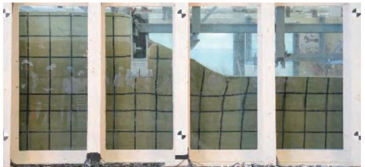
Photo 3 Ground deformation after excitation (Case 1)
