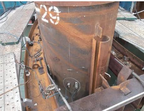
Photo 2 Condition in which sensors are pasted on test pile
