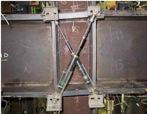
Photo 1 At the stage of maximum strength of peripheral fillet weld of cruciform framing test specimen (fracture of peripheral fillet weld)
