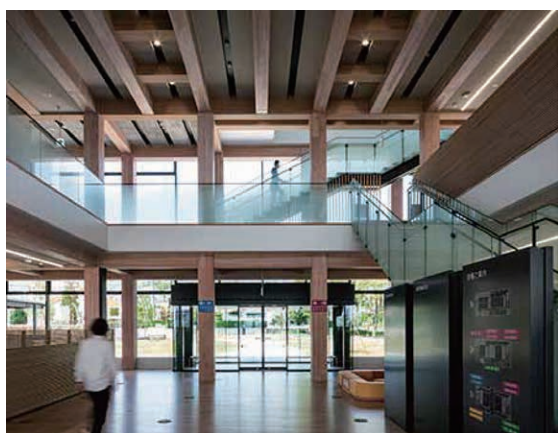
Photo 5 Adoption of wood-steel hybrid structure realizes a large space with a texture like a wooden structure.
