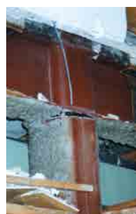
Fracture of weld at column end due to inferior welding
