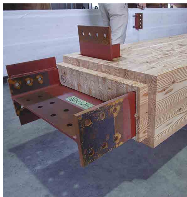
Photo 2 Wood-laminated hybrid member of the steel product built-in type
