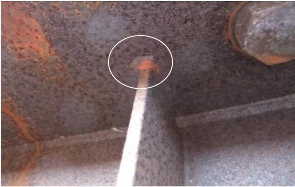
Photo 3 Fatigue crack
