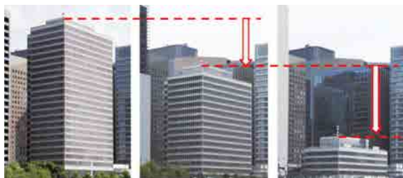
Cut and take down demolition method
