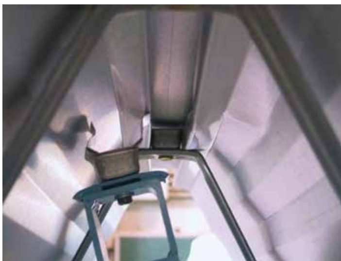
Photo 4 Example of strength test for the connection of folded roofing (SSR2007)
