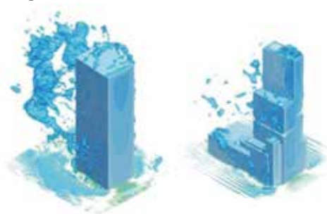
Fig. 1 Statuses of Karman Vortices
