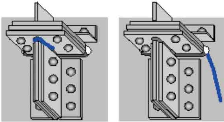
(a) Crack occurring from stringer pedestal (b) Crack occurring from boxing weld zone within slit of cross section
