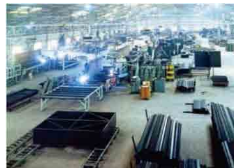
Photo 4 Shop production line of panel-frame system
