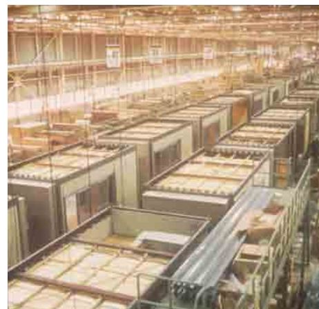
Photo 6 From around 1970, extensive efforts were directed toward developing the structural method that enhances the prefabrication ratio (photo: an example of unit system housing production line).
