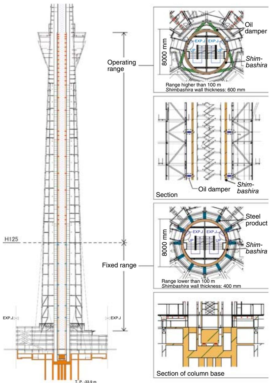
in the foundation structure. The thickness of the steel plate wall was set at 55 mm and 22 mm, and that of the RC wall at 2,700 mm and 1,900 mm.
