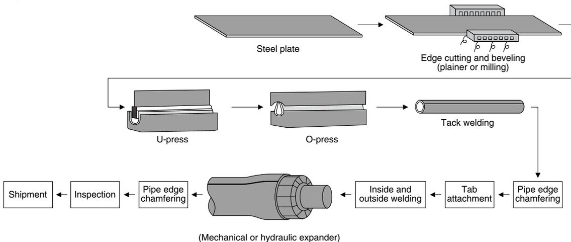
**Fig. 2 Roll-bending or Press-bending Pipe-making Process**
