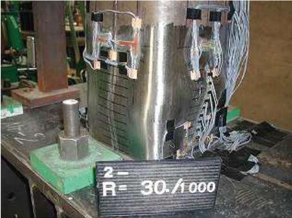
Photo 2 Final test conditions of high-strength CFT columns
