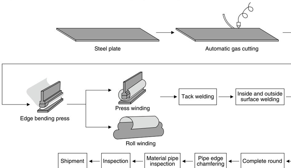
or roll-bending process. Examples of these processes are shown in Figs. 1 and 2.
