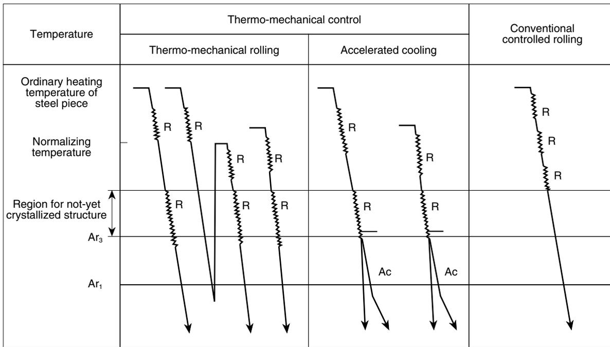
R: Under pressure Ac: Accelerated cooling
