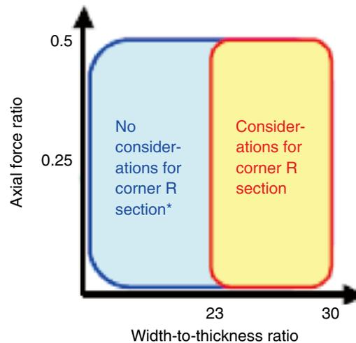
\* In the case of 45°-direction loading, it is necessary to pay due considerations to the shape and material properties of corner R section.
