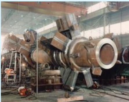
High-performance circular steel tube for the CFT structure
