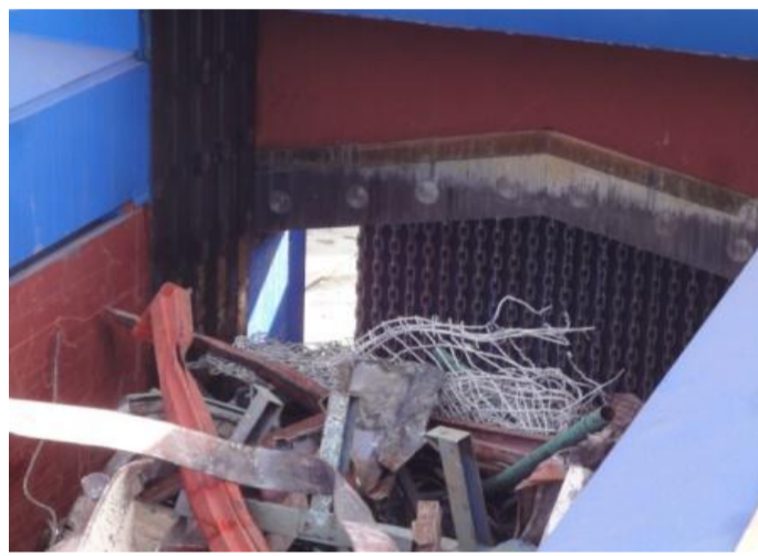
Before scrap pretreatment (0.3 ton/m3)
