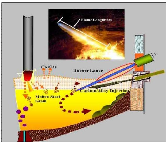
New type of burner has been used to inject carbon and oxygen from side wall and closed slag door. The burner can realize evenly distributed slag-foaming and
