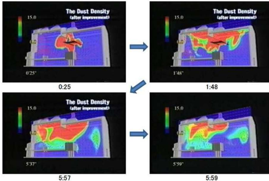
Floating dust density around EAF (by laser-scattering dust indicator)
