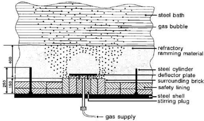
Schematic sketch of gas injection nozzle 2)
