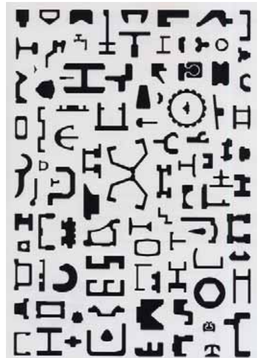
Fig. 1 Sectional Configurations of Hot-extruded Steel Shapes
