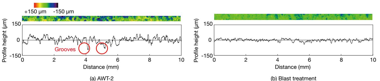
Fig. 4 shows the surface roughness  $R_a$  and  $R_{zjs}$  of the specimens subjected to AWT and blast treatment. The AWT specimen showed a surface roughness about 2 times higher than that of blast-treatment specimens, and as the standoff distance increased, the surface roughness tended to slightly decrease. It was assumed that this was attributable to the fact that the collision energy for the steel substrate of AWT specimens was higher than that of blast-treatment specimens.
