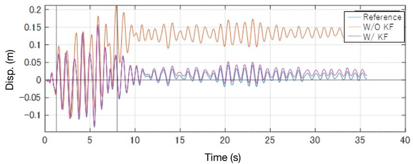
**Table 2 Displacement Estimation Using the Data-driven State-Space Model Identification**
