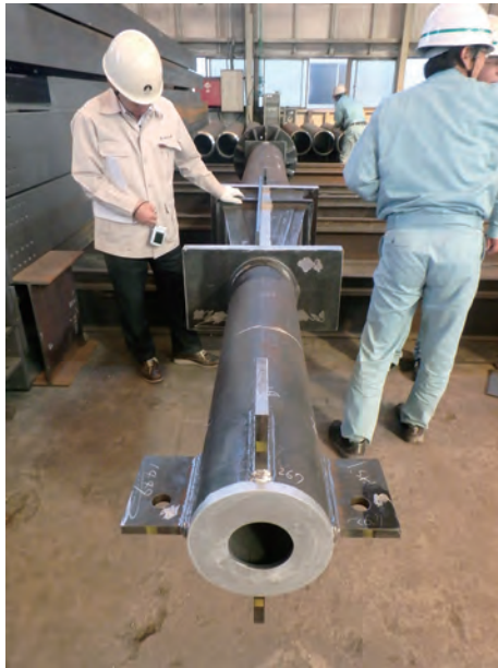
Photo 5 Heavy-wall seamless steel tube used as column
