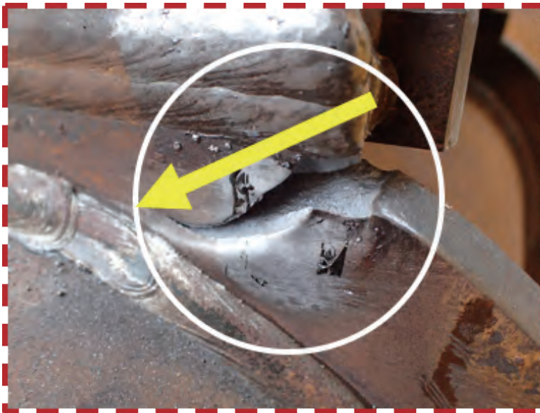
Fig. 7 Fracture of Diaphragm
