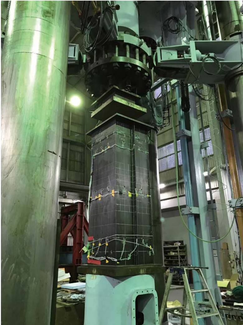
Photo 1 Stiffening plate compressive test specimen prepared using SBHS500 (steel for bridge high-performance structures)
