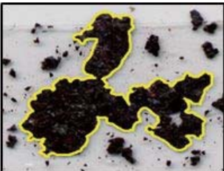
Fig. 3 Overlapped Rust Particles
