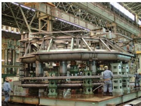
Photo 1 Factory temporary assembly of gate leaf (movable frame) employing SUS821L1
