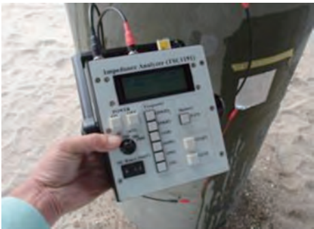
Photo 6 Impedance measurement for painting method
