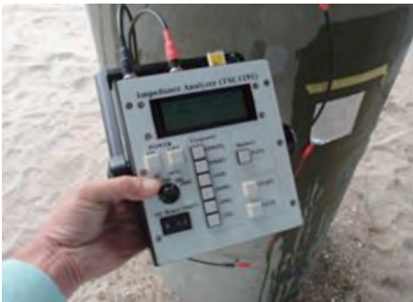
Photo 6 Impedance measurement for painting method
