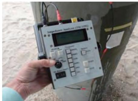
Photo 6 Impedance measurement for painting method
