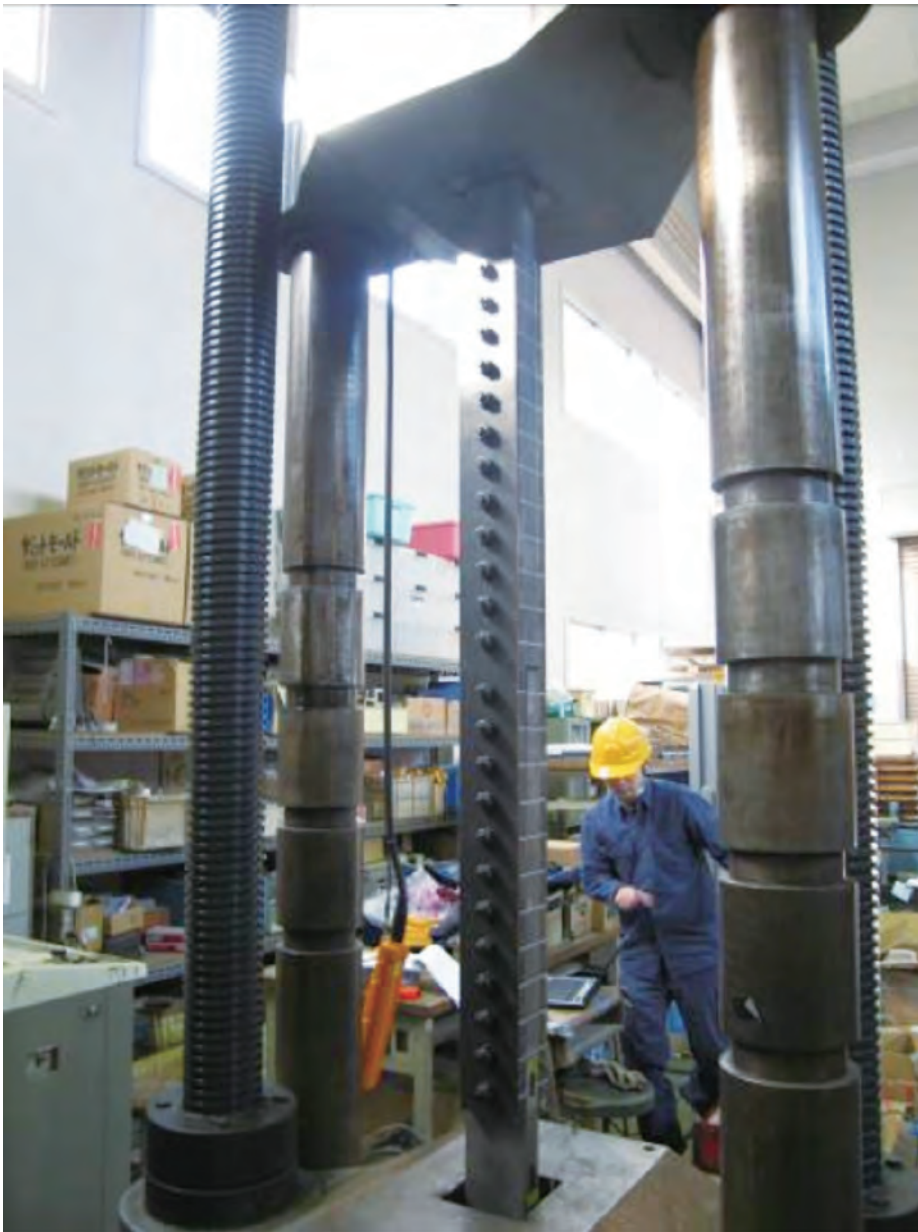
Photo 2 Slip strength test for multiple-row high-strength bolt friction joint with heavier plate thickness
