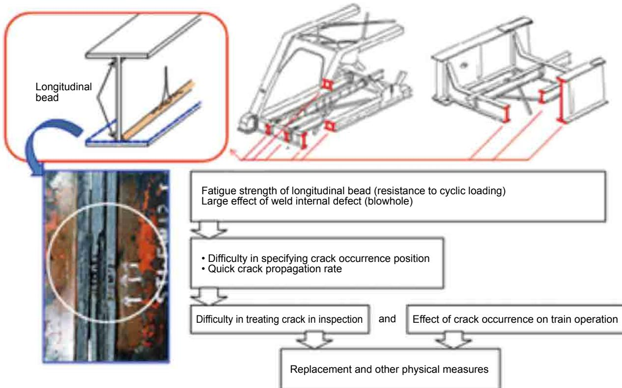
tentionally infused with blowholes (Photo 1). The test results for both the full-scale bridge specimen and the girder specimen satisfy the “Class D” designation prescribed in the fatigue design guidelines of the Japanese Society of Steel Construction and other organizations (Fig. 2). And the developed stress measured in all the steel bridges on the Tokaido Shinkansen falls below the Class D fa-
