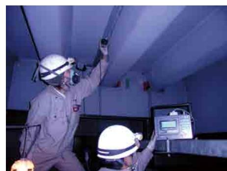
Photo 4 Instrumental inspection (ultrasonic testing of welds of steel structures)
