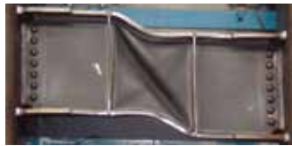
Fig. 1 Example of Ultimate State of Beams with Preceded Shear Yielding (Test Specimen F-1)
