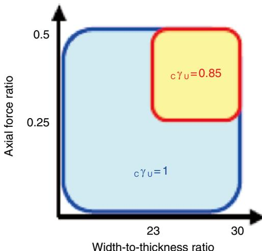
Fig. 2 Treatment of Corner R Section depending on Width-to-Thickness Ratio
