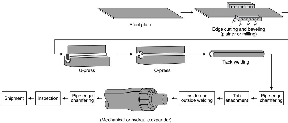
**Fig. 2 Roll-bending or Press-bending Pipe-making Process**
