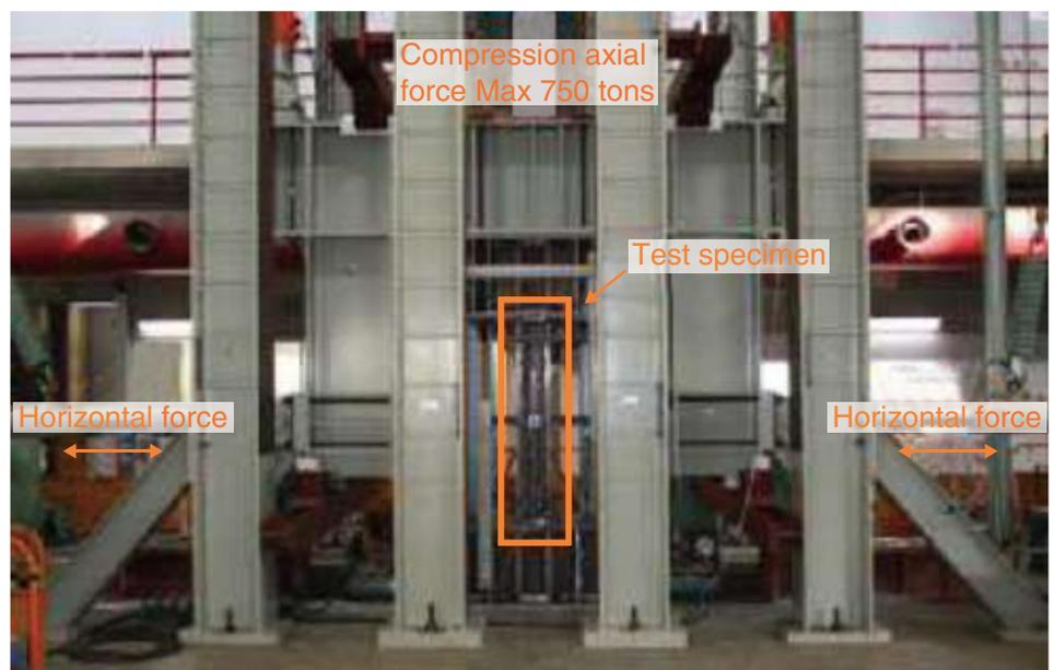
Photo 1 Tests on high-strength CFT columns
